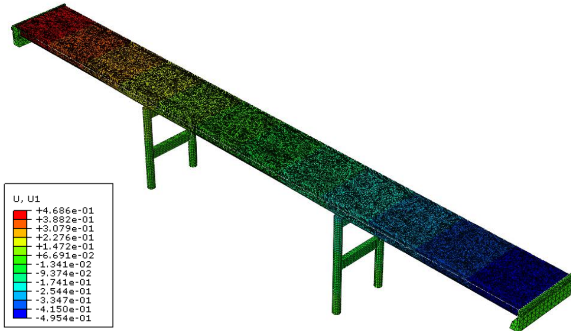
Figure 4.8: Story - Deformation Contour Plot for Temperature Loading
